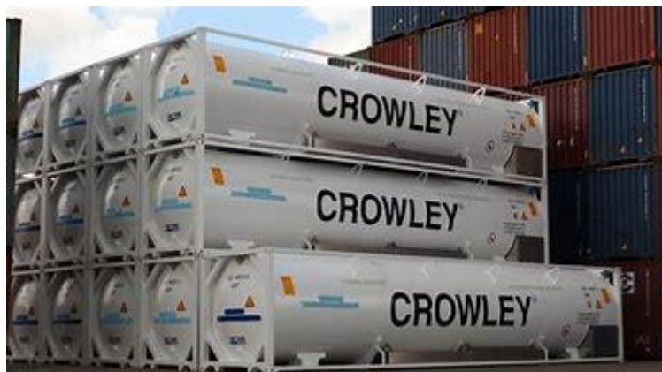
Figure 6 Stockage conteneurs ISO
