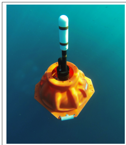
Figure 3. Bombyx 2 with the 4G transmitter and the floatability variation system. The 5 hydrophones array is fixed at the bottom.
